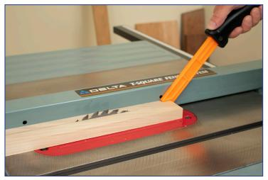
Push sticks are designed to be used on table saws when the stock being cut is too narrow to feed through manually. The notch on the end of the stick helps control and push the stock through the saw blade.
